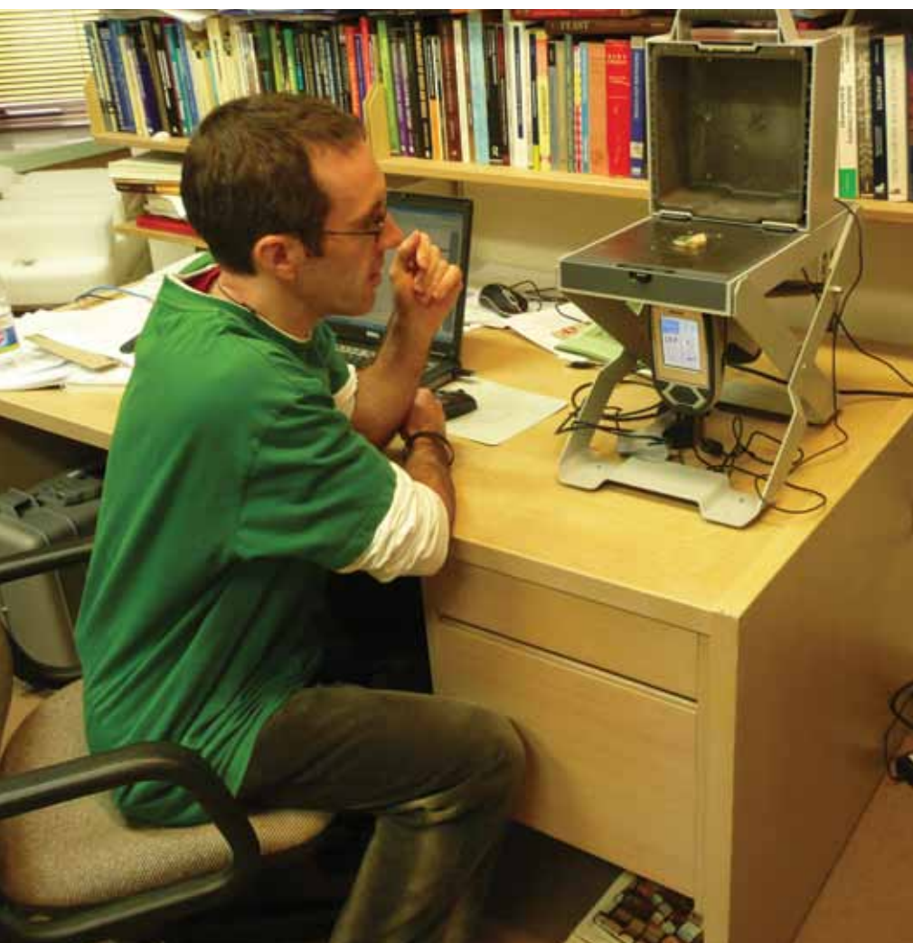
David Thomas using the XRF machine to zap samples and discover their chemical composition (photo: Mark Eccleston).
